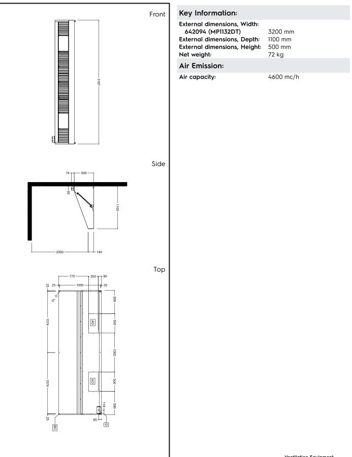
Ventilation Equipment 304 S/S Wall Hood+Filters 3200X1100mm
